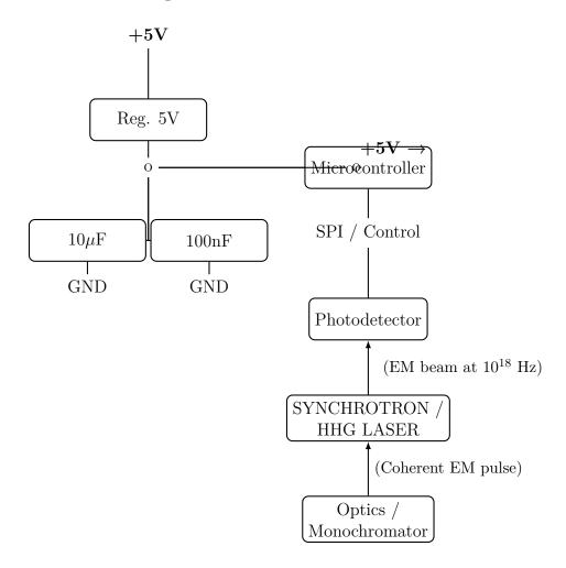
To generate radiation at  $10^{18}$  Hz, one must employ photonic sources (XFEL / synchrotron or HHG driven by femtosecond lasers). The *Optical Source (XFEL/HHG)* block illuminates a photodetector; the detector delivers the electrical signal to the measurement electronics. The **HHG LASER** and the **SYNCHROTRON** constitute the dominant cost.
